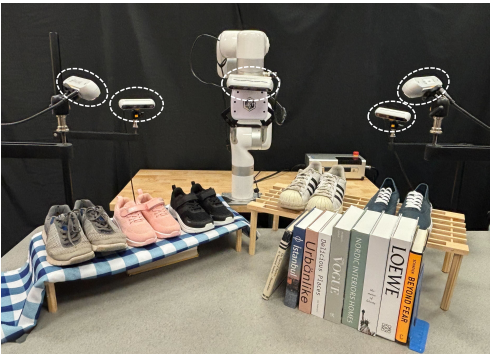
Fig. 4: Setup and experiment objects. We use XArm7 to conduct all our experiments. We use 4 stationary and 1 wrist-mounted camera. We experiment with 5 shoe pairs and 2 shoe racks for tasks involving shoe scenarios. We experiment with 9 different books for stowing tasks.
